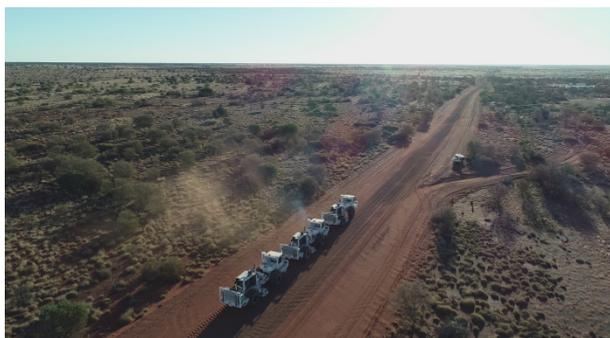
**Figure 2. Vibroseis vehicles in the Kidson Sub-basin taken during the acquisition program (photo credit: Leon Normore, GSWA).**
